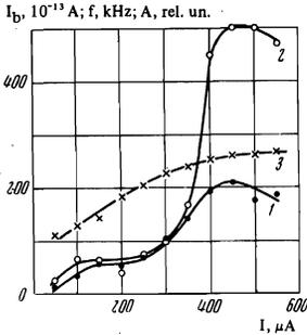
FIG. 3. The probe current  $I_b$  (curve 2) and the amplitude  $A$  (1) and frequency  $f$  (3) of the electron-ion oscillations in the anode current as functions of the beam current  $I$ . Argon,  $p \approx 6 \times 10^{-6}$  mm Hg,  $U_{acc} = 150$  V,  $U_a = 15$  V.
