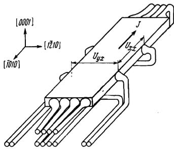
FIG. 1. Mounting of samples for the measurement of the Hall emf and the resistivity.
