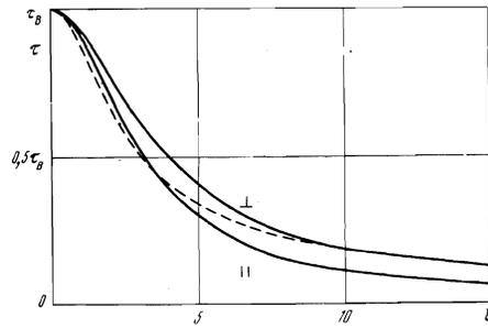
Dependence of relaxation times on dimensionless field  $\xi$ . Solid lines:  $\tau_{1,0}(\parallel)$  and  $\tau_{1,\pm 1}(\perp)$ , calculated by Galerkin's method. These curves are approximated by the functions  $\tau_{\parallel}$  and  $\tau_{\perp}$  of (28) with accuracy 15% ( $\parallel$ ) and 7% ( $\perp$ ). Dotted lines:  $\tau_{\perp}$  from (30).
