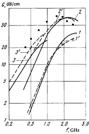
FIG. 2. Dependence of the electronic gain of ultrasound on the frequency for fixed drift velocity of the electrons:  $\circ$  --  $v_d/v_s = 30$ ;  $\bullet$  --  $v_d/v_s = 170$ . Solid curves -- theoretical. 1 -- according to [3], 1' -- according to [11],  $v_d/v_s = 30$ ; 2 -- according to [3]; 2' -- according to [11],  $v_d/v_s = 170$ ; 3 -- according to [12]; 3' -- according to [13],  $v_d/v_s = 170$ .
