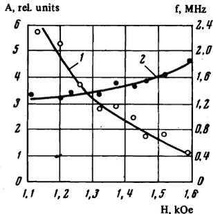
FIG. 5. Amplitude (1) and frequency (2) of oscillations as functions of the magnetic field. Helium gas, beam energy 4.2 keV,  $p = 6.5 \times 10^{-4}$  mm Hg ( $A = 1$  corresponds to noise level).
