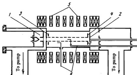
FIG. 2. Schematic illustration of the experimental setup: 1—ion source, 2—ion beam collector, 3, 4—diaphragms, 5—magnetic field coils, 6—probes.
