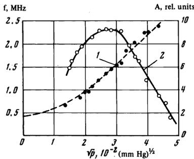
FIG. 4. Oscillation frequency at maximum amplitude as a function of pressure (curve 1, broken line represents theoretical prediction) and dependence of the oscillation amplitude on the helium gas pressure in the chamber (curve 2). Beam energy 5 keV,  $H_0 = 1.1$  kOe.
