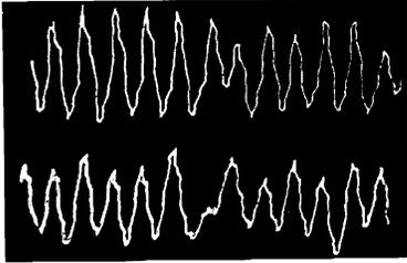
FIG. 6. Oscillations of the magnetic flux in the sample (upper curve) and oscillations of the resistance (lower curve). Sample 2,  $T = 3.24^\circ\text{K}$ ,  $H_e = 0.18 H_C = 4.5 \text{ Oe}$ ,  $I = 1.05 \text{ A}$  and  $I_C = 44 \text{ A}$ . The oscillation frequency is 10 Hz. The amplitude of the magnetic-flux oscillations is  $\sim 4\%$  of the average value of the magnetic flux in the sample. The amplitude of the oscillations of the resistance is  $\sim 2\%$  of the average value.
