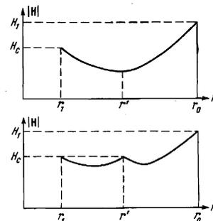
FIG. 1. Distribution of the magnetic field in the normal metal outside the TM-state layer before the nucleation of the s layer (above) and after the nucleation (below).
