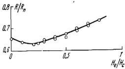
FIG. 5. Jump of sample resistance at  $I = I_C$  as a function of the external magnetic field. Sample 2,  $T = 3.24^\circ\text{K}$ .
