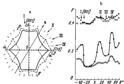
FIG. 4. Orientation of sample In4 (a) and dependences of the helicon damping on the angle between the external magnetic field  $H_0$  and the vector  $k$ :  $\circ$ — $f = 181$  Hz,  $\lambda \approx 1.4$  mm;  $\bullet$ — $f = 1616$  Hz,  $\lambda \approx 0.47$  mm. The upper two curves correspond to  $T = 4.2^\circ$  K and the lower two curves to  $T = 1.35^\circ$  K.
