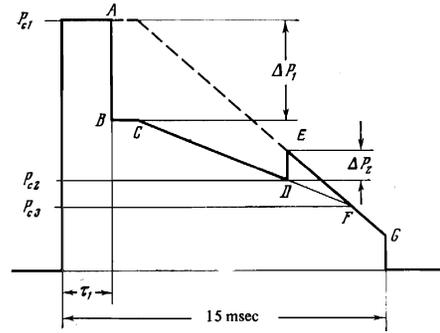
FIG. 6. Schematic representation of the non-rectangular pulse whose oscillogram is shown in Fig. 2b.
