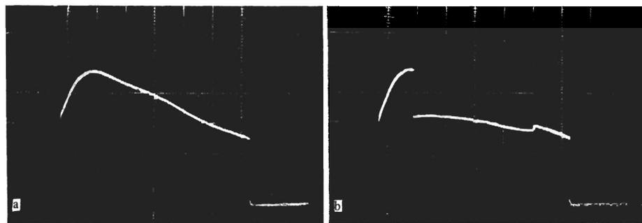
FIG. 2. Oscillograms of pulses: a—Pulse passing through resonator in the absence of beyond-threshold absorption in the sample. b—Pulse in the presence of such absorption.
