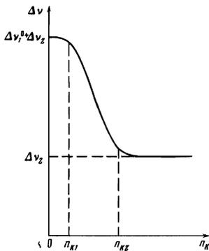
FIG. 5. Proposed dependence of the relaxation  $\Delta\nu$  on the spin-wave density  $n_k$ .
