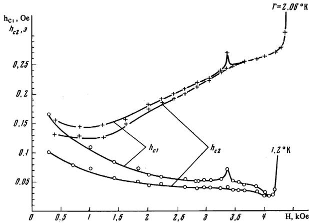
FIG. 4. Dependence of the critical fields  $h_{c1}$  and  $h_{c2}$  on the static field  $H$ .
