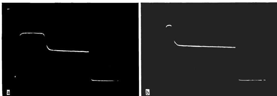
FIG. 1. Oscillograms of rectangular pulse passing through the resonator in the presence of beyond-threshold absorption in the sample: a— $\tau_1 = 80 \mu\text{sec}$ ; b— $\tau_1 = 20 \mu\text{sec}$ .
