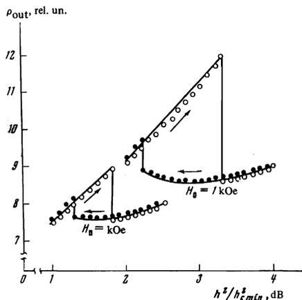
FIG. 2. Sample plots of the transmitted power against the power at the resonator input at fixed  $H_0$ . (All the powers were measured relative to the minimum threshold value,  $h_{c \min} \approx 0.1$  Oe). The designations of the points are the same as in Fig. 1b.
