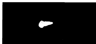
FIG. 2. Photograph of a spark in optical breakdown of CO_2 at p = 1 atm.
