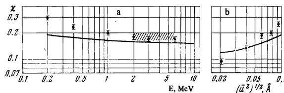
FIG. 2. Minimal yield (a) as a function of incident-particle energy and (b) as a function of thermal-vibration amplitude of the atoms. The cross-hatched region represents the experimental results<sup>[12]</sup>. The points show the results of computer calculation<sup>[7]</sup>.
