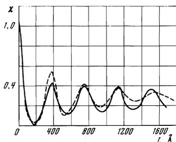
FIG. 1. Behavior of the minimal yield of a nuclear reaction near the surface of a single crystal. The solid line is the theoretical curve, and the dashed line is the curve obtained by the Monte Carlo method<sup>[7]</sup>.
