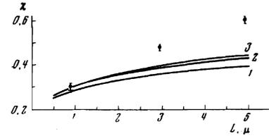
FIG. 3. Plane dechanneling: 1—yield curve without inclusion of electron collisions, 2—with inclusion of electron collisions, 3—with inclusion of stopping. The experimental points were taken from ref. 12.
