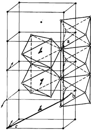
FIG. 1. Relationship between the rutile (TiO<sub>2</sub>) structure and the structures of MoO<sub>2</sub> and WO<sub>2</sub>: ●—metal; ○—oxygen.
