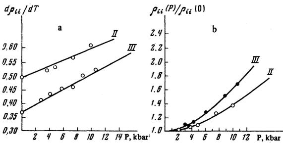
FIG. 1. a—Pressure dependence of the temperature coefficient  $d\rho_{ii}/dT$  in Sb,  $T = 77-120^\circ\text{K}$ , II— $d\rho_{22}/dT$ , III— $d\rho_{33}/dT$ . The ordinates represent the slope of  $\rho_{ii}(\Omega\text{-cm})$  with respect to  $T$ . b—Relative pressure variation, at  $T \sim 83^\circ\text{K}$ , of the resistivity  $\rho_{ii}(P)/\rho_{ii}(0)$ . Curves II— $\rho_{22}(P)/\rho_{22}(0)$ , III— $\rho_{33}(P)/\rho_{33}(0)$ .
