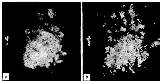
FIG. 4. Electron (a) and ion (b) field emission pictures of a crystal bombarded at  $21^{\circ}\text{K}$ .
