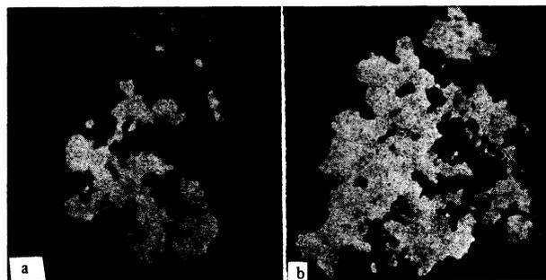
FIG. 2. Broadening of ion field emission image of bombarded tungsten microcrystal: a—microgram taken immediately after bombardment, b—after deformation at  $\sigma \approx 500$  kgf/mm<sup>2</sup>.
