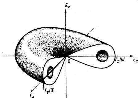
FIG. 1. Boundary surface  $p = 0$ . Motion along the line  $0-E_y(0)-0$  corresponds to a self-focusing waveguide of the TE type; motion along the loop  $0-E_x(0)-0$  formed by intersection of the boundary surface by the plane  $E_y = 0$  corresponds to a waveguide of the TM type.
