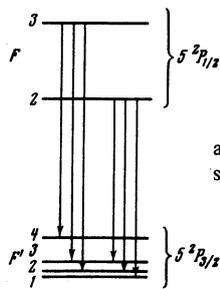
FIG. 1. Hyperfine splitting of the iodine atom levels  $5^2P_{1/2}$  and  $5^2P_{3/2}$ . The arrows show the possible radiative transitions.
