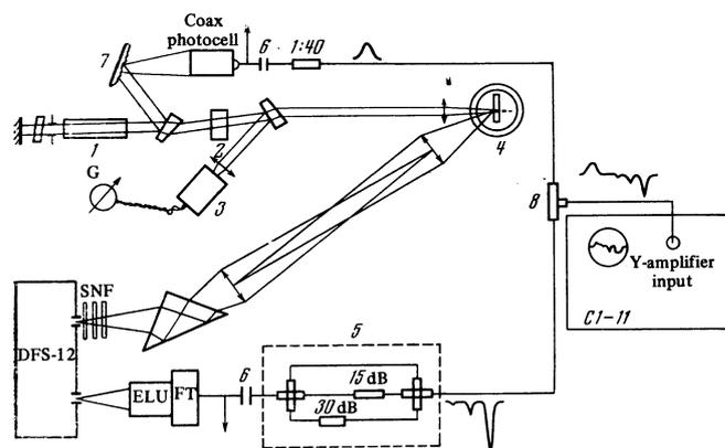
FIG. 1. Diagram of experimental setup: 1—laser, 2—cell with  $\text{CuSO}_4$  solution in water, 3—thermoelectric calorimeter, G—control galvanometer, 4—cell with investigated powder, placed in a Dewar, 5—attenuation for extending the dynamic range of the oscilloscope, 6—voltage-dividing capacitors, 7—scattering surface, 8—splitter.
