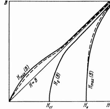
Fig. 2—Stability limits of mixed state  $H_{min}(B)$  and  $H_{max}(B)$  (shown schematically). The solid lines pertain to the case of Fig. 1a and the dashed to the case Fig 1b.  $H_0(B)$  is the equilibrium magnetization curve.
