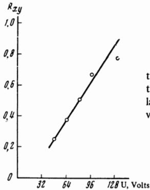
FIG. 6. Correlation coefficient between oscillations of the ion current and the signal from the output of the modulation generator as a function of the voltage of the latter.
