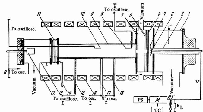
FIG. 1. Block diagram of apparatus: 1—electron gun chamber; 2—electron gun; 3—cathode; 4—grid; 5—anode; 6 and 7—two pairs of diaphragms; 8 and 10—internal probes; 9—plasma chamber; 11—syphon bellows; 12—Faraday cylinder; 13—experimental chamber; 14—leak valve; 15—external probes; 16—magnetic field coil; 17 and 18—ten- and three-centimeter waveguides; PS—power supply; M—modulator; TC—trigger circuit.
