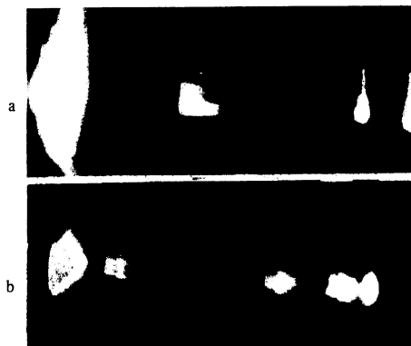
FIG. 3. Ultrashort pulses before (a) and after (b) passage through a cuvette containing a solution of vanadium phthalocyanine in nitrobenzene. The axial period was 20 nsec. The separation between pulses formed by mirrors R_2 and R_3 was 0.1 nsec.
