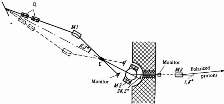
FIG. 2. Method of producing the polarized proton beam.
