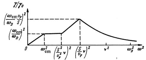
FIG. 1. Frequency dependence of the transformation coefficient for  $l \ll \delta_0$ .
