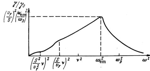
FIG. 4. Frequency dependence of the transformation coefficient for  $\delta_0(v_F/s)^{3/2} \ll l$ .
