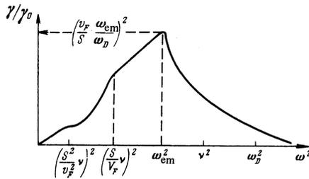
FIG. 3. Frequency dependence of the transformation coefficient for  $\delta_0(v_F/s)^{1/2} \ll l \ll \delta_0(v_F/s)^{3/2}$ .
