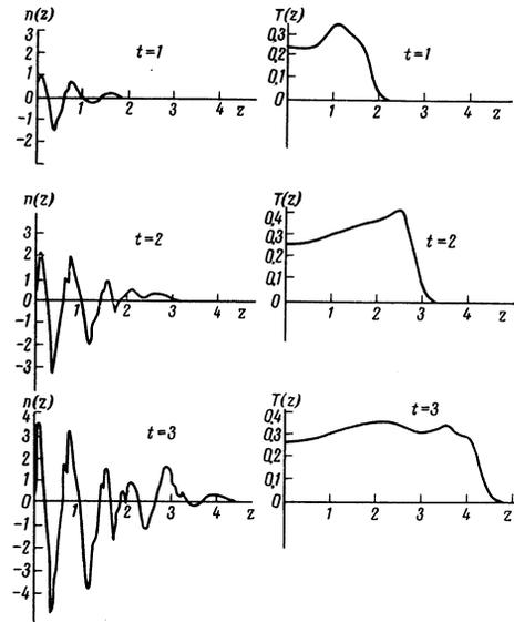
FIG. 2. Plasma temperature and concentration profiles in a one-dimensional relaxation wave. The dimensionless variables introduced in Sec. 4 are used, and  $\chi = 1/10$ .
