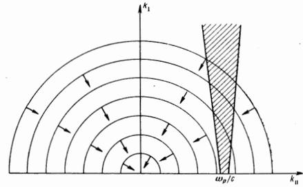
FIG. 1. Illustrating the theory of relaxation of an ultrarelativistic beam in a plasma. The wave-vector region in which there is interaction between the oscillations and the beam is shown shaded. The concentric circles represent the lines along which isotropization of the oscillation spectrum takes place. The arrows indicate the direction of the spectral transfer.
