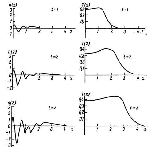
FIG. 3. Plasma temperature and concentration profiles in a one-dimensional relaxation wave,  $\chi = 1/3$ .
