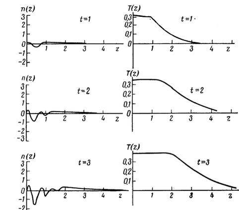
FIG. 4. Plasma temperature and concentration profiles in a one-dimensional relaxation wave,  $\chi = 1$ .
