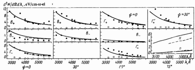
FIG. 3. Spectral distribution of radiation density for Al ( $\Gamma_{+}a = 384\text{\AA}$ ,  $B_{-}a = 272\text{\AA}$ ) for  $E = 40\text{ keV}$ :  $\bullet - W_{\parallel}$ ,  $\circ - W_{\perp}$ . Backward radiation:  $B_{-}\theta = 127.5^{\circ}$ ;  $\Gamma_{+}\theta' = -52.5^{\circ}$ ;  $\Gamma_{+}'\theta' = 52.5^{\circ}$ .
