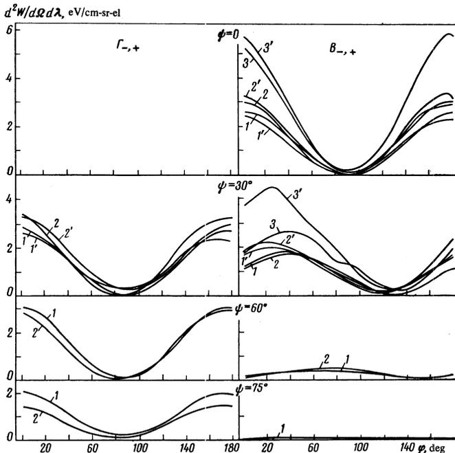
FIG. 1. Spectral density of radiation as a function of the angle  $\varphi$ .  $E = 80$  keV,  $\lambda = 5000 \text{ \AA}$ . Backward radiation: 1—Au,  $a = 400 \text{ \AA}$ ; 2—Cu,  $a = 674 \text{ \AA}$ ; 3—Al,  $a = 272 \text{ \AA}$ ;  $B_- - \theta = 127.5^\circ$ ,  $\Gamma_- - \theta' = -52.5^\circ$ . Forward radiation: 1'—Au,  $a = 400 \text{ \AA}$ ; 2'—Cu,  $a = 674 \text{ \AA}$ ; 3'—Al,  $a = 272 \text{ \AA}$ ;  $B_+ - \theta = 52.5^\circ$ ;  $\Gamma_+ - \theta' = -52.5^\circ$ .
