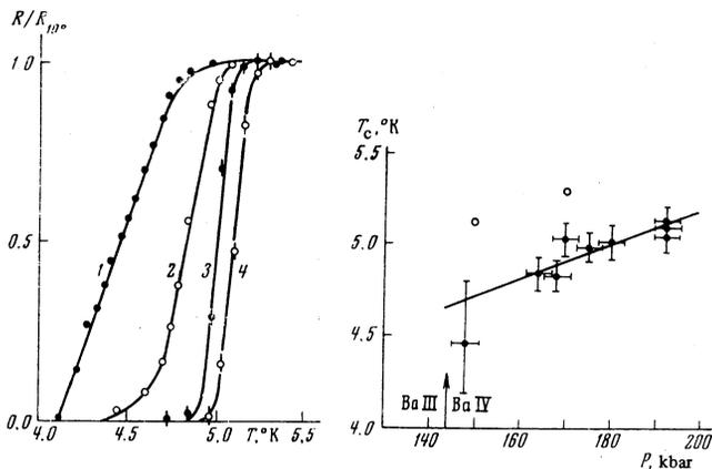
FIG. 3. Curves of the superconducting transitions in barium for various pressures  $P$  (kbar): 1—148, 2—168, 3—175, 4—192.
