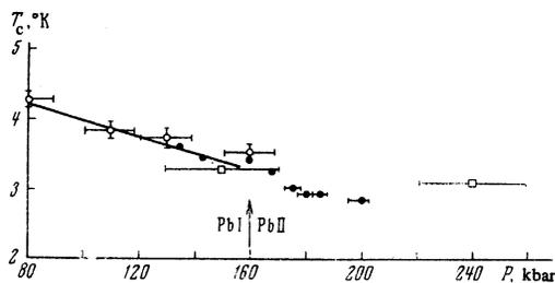
FIG. 6. Plot of  $T_C(P)$  for lead:  $\circ$ —data of [5],  $\square$ —[8],  $\bullet$ —present work.
