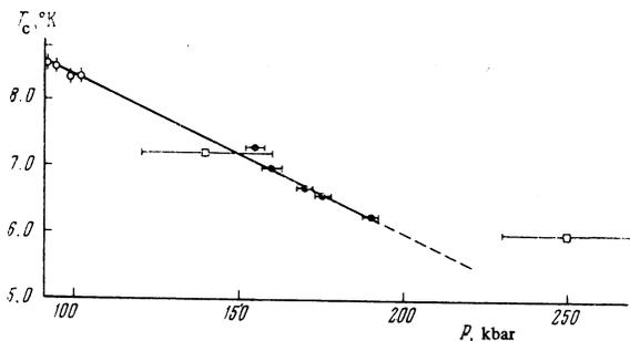
FIG. 2. Dependence of  $T_c(P)$  for the high pressure modification Bi IV:  $\circ$ —data of [7],  $\square$ —[8],  $\bullet$ —present work.
