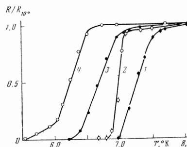
FIG. 1. Curves of the superconducting transition in bismuth at various pressures  $P$  (kbar): 1–153, 2–160, 3–170, 4–190.
