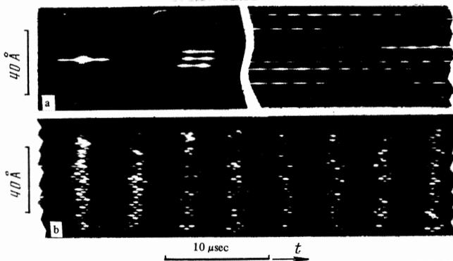
FIG. 6. Time scan of generation spectrum with moving misaligned selector;  $a_2 = 2$  mm,  $v = 25$  cm/sec; a) misalignment  $1.5''$ ; b) misalignment  $40''$ .
