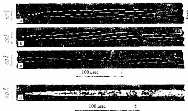
FIG. 4. Time scan of generation spectrum. Diaphragm of 1.5 mm diameter; a) selector omitted; b, c) selector fixed ( $a_2 = 10$  mm); d) selector moving,  $v = 25$  cm/sec.
