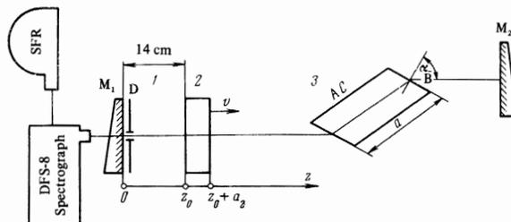
FIG. 1. Diagram of the experimental setup. M1, M2—plane mirrors of resonator; AM—active medium; a—length of active medium.
