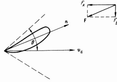
FIG. 1. Directivity pattern of phonon radiation and direction of electroacoustic force in a crystal where the phonon generation intensity is maximal in the direction of the vector  $\mathbf{n}$ . The Cerenkov angle  $\theta$  is determined by the condition  $\cos \theta = v^\alpha / v_d$ .
