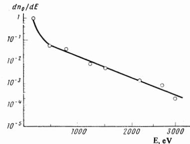
FIG. 1. Energy spectrum of neutral charge-exchange atoms,  $T_i = 390 \text{ eV}$ .
