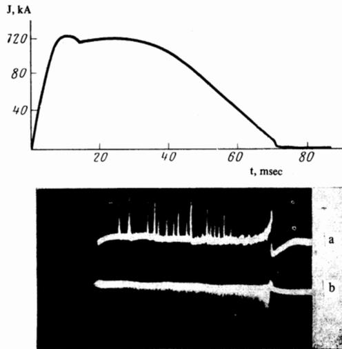
FIG. 2. Oscillogram of signals of boron (a) and scintillation (b) counters; top—oscillogram of discharge current on the same time scale.
