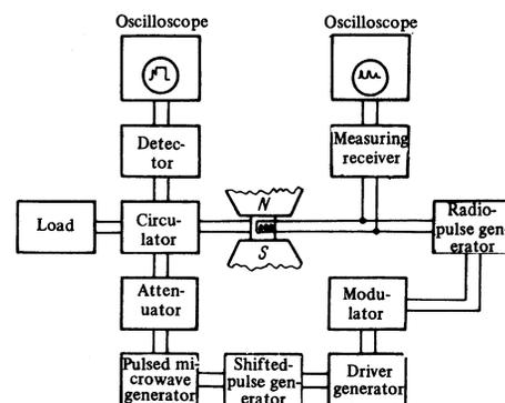
FIG. 1. Block diagram of experimental setup. The programmed generator, modulator, radio-pulse generator, measuring receiver, and oscilloscope compose the nuclear-spin-echo spectrometer, and the rest of the equipment is the apparatus for excitation of parametric spin waves.
