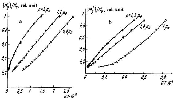
FIG. 4. Dependence of  $|M'_g|/M_0|_{T=\text{const}}$  on  $QT$  for samples of nickel and iron for different values of the parameter  $p$ : a—nickel,  $T = 0.9^\circ\text{K}$ ; b—iron,  $T = 1^\circ\text{K}$ .
