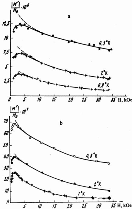
FIG. 2. Dependence of the quantity  $|M'/M_0|_{T=\text{const}}$  on magnetic field for nickel (a) and iron (b) samples ( $M' \equiv \partial M/\partial T$ ) for different temperatures. The averaged dependence of  $|M'/M_0|$  on  $H$  is shown by solid lines. The dependence of  $|M'_g/M_0|$  on  $H$  is given by the dashed lines.
