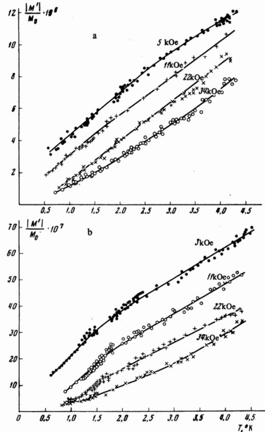
FIG. 3. Dependence of  $M'/M_0|_{H=\text{const}}$  on temperature for nickel (a) and iron (b) samples in different magnetic fields. The solid lines are averaged from several experiments.
