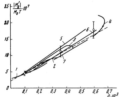
FIG. 6. Dependence of the quantities  $\mathcal{M}|_{H=\text{const}}$  and  $\mathcal{M}|_{T=\text{const}}$  on  $Q$  for iron: 1— $H = 34$  kOe, 2—22 kOe, 3—11 kOe, 4—3 kOe (the arrows show the direction of increasing temperature); 5— $T = 1^\circ\text{K}$ , 6— $2^\circ\text{K}$ , 7— $4.3^\circ\text{K}$ . The dashed line is drawn for calculation of the constants  $C$  and  $2A/M_0$ . The maximum possible random error is indicated.
