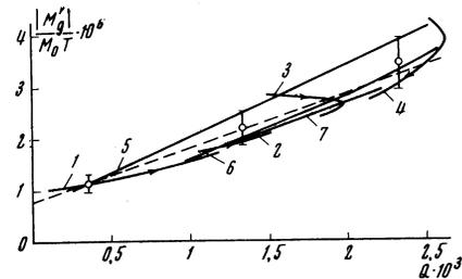
FIG. 5. Dependence of the quantities  $\mathcal{M}|_{H=\text{const}}$  and  $\mathcal{M}|_{T=\text{const}}$  on  $Q$  for nickel ( $\mathcal{M} \equiv |M'_g|/M_0 T$ ): curve 1— $H = 34$  kOe; 2—22 kOe; 3—11 kOe; 4—5 kOe (the arrows indicate direction of increasing temperature curve 5— $T = 0.9^\circ\text{K}$ , 6— $2^\circ\text{K}$ , 7— $4.3^\circ\text{K}$ ). The dashed line is drawn for calculation of the constants  $C$  and  $2A/M_0$ . The maximum possible random error is indicated.
