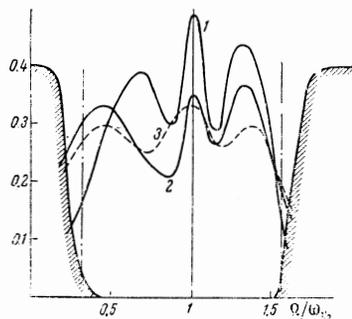
FIG. 3. Noise spectrum of the hf discharge (relative units) obtained by correlation analysis of magnetic probe output: 1— $H_Z = 1.5$  kOe, 2— $H_Z = 4$  kOe, 3— $H_Z = 6$  kOe;  $\Omega = \omega_{1/2}$ —frequency of paramagnetic instability.
