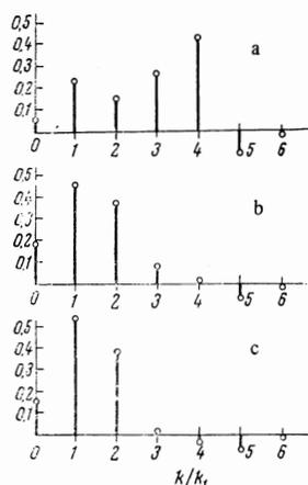
FIG. 4. Spectrum of spatial harmonics of the instabilities (relative units) with  $\Omega = \omega_{1/2}$  for different fields  $H_Z$ : a—1 kOe, b—2 kOe, c—3 kOe.
