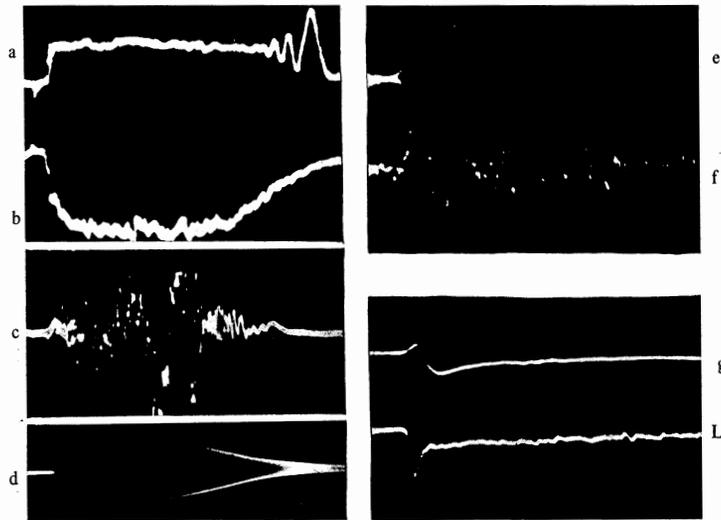
FIG. 1. a—Output of the 2.26-mm interferometer, b—intensity of the continuum between 5700 and 5750Å, c—reflected 2.26-mm signal, d—signal of the Rogowski loop measuring the current in the plasma, e—magnetic probe output, f—rectified magnetic probe output, g—low-frequency component of the diamagnetic probe, h— $H_{\beta}$ . Time scale a–d 500  $\mu$ sec, e–h 200  $\mu$ sec.
