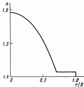
FIG. 5. The index of refraction of a lens with a homogeneous external layer which focuses a parallel beam of rays on its own surface.
