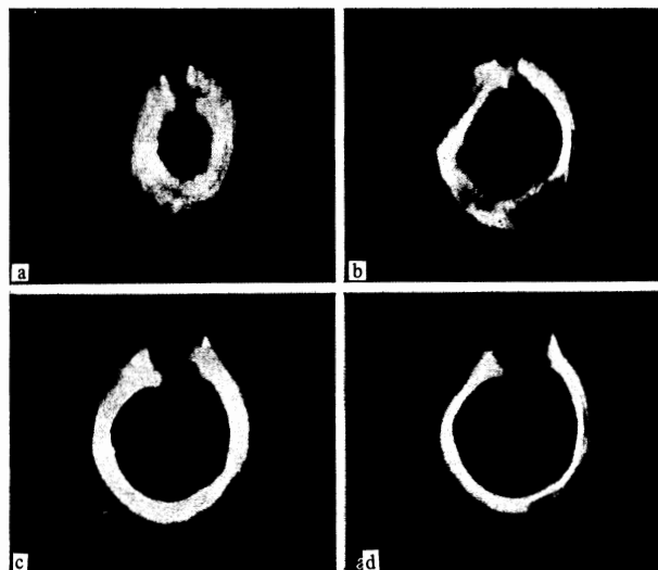
FIG. 1. Expansion of shadow from a small body in water (beam passed horizontally) at various times: a— t = 0 , b— t = 3 sec, c— t = 5 sec, d— t = 10 sec.
