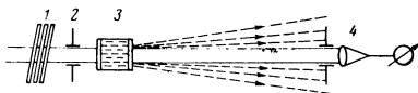
FIG. 3. Diagram of experiment for the study of nonlinear losses in nitrobenzene: 1—neutral light filters, 2—diaphragm, 3—cell with 7-cm nitrobenzene layer, 4—calorimeter.
