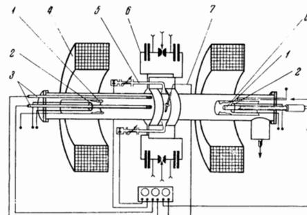
FIG. 1. Diagram of the "Dimpol" setup: 1—anode of Penning discharge, 2—cathodes, 3—magnetic probes, 4—coils of constant magnetic field, 5—microwave-noise pickups, 6—high-frequency circuit, 7—radial magnetic probe, 8—pickup for bremsstrahlung x-radiation from the target.
