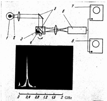
FIG. 2. Diagram of the setup for the analysis of oscillations recorded on the oscilloscopes: 1—light source, 2—ground glass, 3—oscillogram pattern, 4—cylinder of organic glass, 5—mirror, 6—photomultiplier, 7—oscilloscope for controlling the form of the oscillations, 8—spectrum analyzer ASChKh-1.
