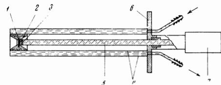
FIG. 3. Scintillation pickup for bremsstrahlung x rays from the target: 1—target, 2—absorber-filter, 3—scintillator CsI(Tl), 4—cooled screen, 5—lightpipe, 6—flange, 7—FEU-13 photomultiplier.
