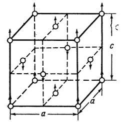
FIG. 7. Magnetic structure of  $\gamma$ -Mn.
