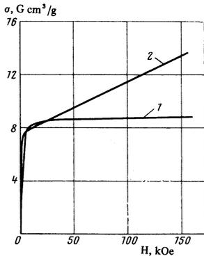
FIG. 5. Magnetization curves for a sample of  $\text{Mn}_{0.8}\text{Ge}_{0.2}$  in a high magnetic field: 1—77°K; 2—313°K.
