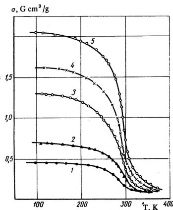
FIG. 4. Temperature dependence of the magnetization of a sample of  $\text{Mn}_{1-x}\text{Ge}_x$  after a two-hour anneal at 920°K: 1— $x = 0.1$ ; 2— $x = 0.14$ ; 3— $x = 0.16$ ; 4— $x = 0.18$ ; 5— $x = 0.20$ .
