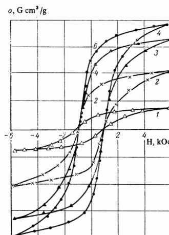
FIG. 1. Effect of heat treatment on the magnetic properties of a sample of  $Mn_{0.8}Ge_{0.2}$ . Temperature of anneal 670°K, time for the different curves: 1–10, 2–30, 3–100, 4–300 h.
