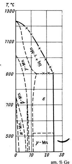
FIG. 8. Possible phase diagram for the Mn-Ge system.
