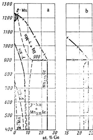
FIG. 6. Phase diagrams of the Mn-Ge system: a—according to [13]; b—according to [16].
