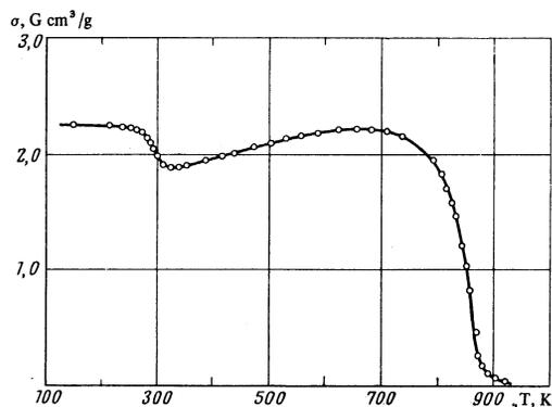
FIG. 2. Temperature dependence of the magnetization of a sample of  $\text{Mn}_{0.84}\text{Ge}_{0.16}$ .
