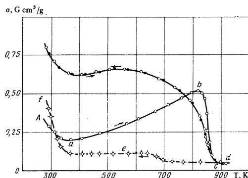
FIG. 3. Change of the temperature dependence of magnetization of a sample of  $\text{Mn}_{0.86}\text{Ge}_{0.14}$  for successive measurement cycles:  $\circ$ —first cycle,  $\bullet$ —subsequent cycles;  $\diamond$ —after heating at 920°K.
