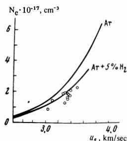
FIG. 5. Dependence of the electron concentration  $N_e$  behind the reflected wave on the velocity of the incident shock wave.
