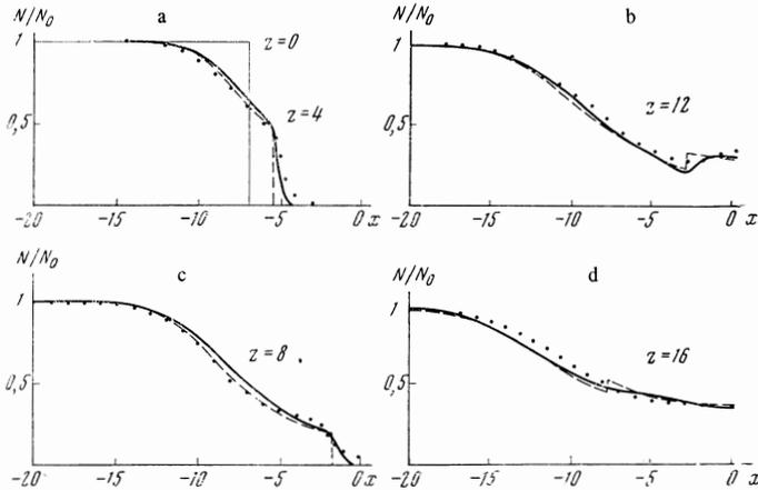
FIG. 5. Concentration of ions behind a plate with  $R = 7D$  as a function of x for different z. Points—experiment; dashed lines ( $T_e/T_i = \infty$ ) and solid lines ( $T_e/T_i = 20$ )—calculation.
