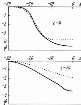
FIG. 6. Potential of plasma behind a plate with  $R = 20D$  as a function of x for different z. Points—experiment; solid curve—calculation ( $T_e/T_i = \infty$ ).
