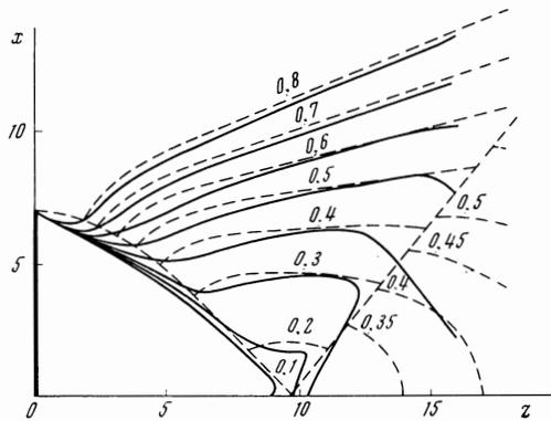
FIG. 1. Surfaces of constant concentration (numbers on the curves) of ions in the case of flow around a plate: dashed curves— $T_e/T_i = \infty$ ; solid curves— $T_e/T_i = 20$ .
