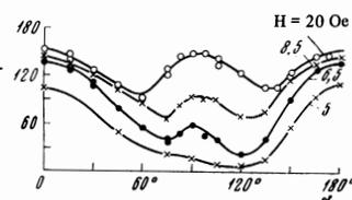
FIG. 1. Dependence of the magneto-optical signal (mV) on the angle of rotation of sample 1 in an external magnetic field.
