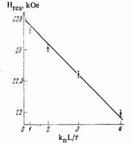
FIG. 5. Resonance fields for various spin-wave modes in sample 1 ( $f = 9.25 \text{ GHz}$ ,  $M = 1600 \text{ G}$ ,  $L = 1240 \pm 70 \text{ \AA}$ ).
