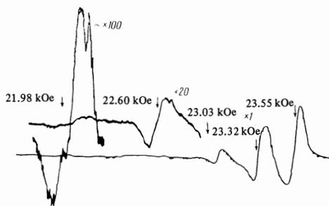
FIG. 2. Spin-wave resonance spectrum of sample 1 in the perpendicular configuration at  $f = 9.25$  GHz. The arrows indicate the resonance peak positions.
