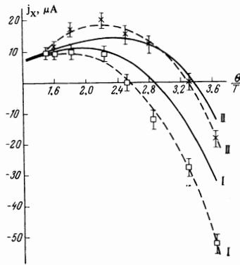
FIG. 3. Temperature dependences of the short-circuit current  $j_x$  in a magnetic field. The dashed curves are the plots of the experimental results and the continuous curves are theoretical. I)  $H_0 = 0$ ; II)  $H_0 = 15$  kOe.
