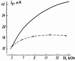
FIG. 7. Dependence of the transverse current  $j_y$  on the magnetic field in the case of open longitudinal contacts. The dashed curve is the plot of the experimental results and the continuous curve is theoretical.  $T = 77^\circ\text{K}$ .
