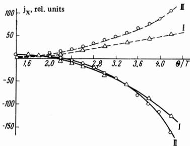
FIG. 4. Calculated temperature dependences of the longitudinal light- and heavy-hole currents. The dashed curves represent the light-hole current  $j_x^{(1)}$  and the continuous curves the heavy-hole current  $j_x^{(2)}$ . I)  $H_0 = 0$ ; II)  $H_0 = 15$  kOe.
