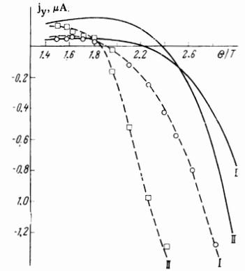
FIG. 5. Temperature dependences of the transverse current  $j_y$  in the case of closed longitudinal contacts. The dashed curves are the plots of the experimental results and the continuous curves are theoretical. I)  $H_0 = 5$  kOe; II)  $H_0 = 13$  kOe.
