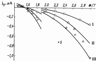
FIG. 6. Temperature dependences of the transverse current  $j_y$  in the case of open longitudinal contacts.  $\square$ )  $H_0 = 3$  kOe;  $\Delta$ )  $H_0 = 7$  kOe;  $\circ$ )  $H_0 = 15$  kOe. I, II, and III are the theoretical curves for  $H_0 = 3$ , 7, and 15 kOe, respectively.
