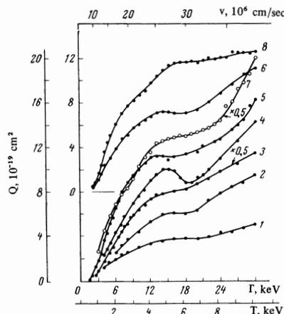
FIG. 1. Cross sections for the excitation of K II lines: 1-λ = 4135, 2-4505, 3-4223/6, 4-3898, 5-4305/9, 6-4596 + 4608, 7-4263, 8-4186 Å, v-K<sup>+</sup> velocity (lab system), T-K kinetic energy, E-energy of relative motion. The origin was shifted for curves 6 and 8.
