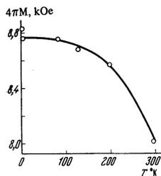
FIG. 10. Temperature dependence of the magnetization of Permalloy, calculated on the assumption that the formula  $(\omega/\gamma)_{\parallel} = H + 4\pi M$  is valid.
