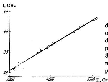
FIG. 9. Frequency dependence of the FMR line position of Permalloy. The straight line drawn through the experimental points obeys Eq. (9) if  $4\pi M = 8070$  Oe and  $g = 2.17$ . The magnetic field was parallel to the plane of the sample.
