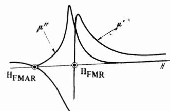
FIG. 1. Dependences of  $\mu'$  and  $\mu''$  on the external magnetic field for  $\omega/\gamma > 4\pi M$ .
