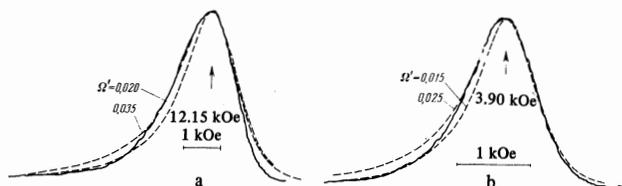
FIG. 6. Experimentally observed ( $f = 36.2$  GHz,  $d = 14 \mu$ ) and calculated (dashed curves;  $\Omega = 1.5$ ,  $d/\delta_0 = 10$ ) antiresonance lines of a Permalloy plate: a) magnetic field perpendicular to the plane of the plate; b) magnetic field parallel to the plane of the plate.
