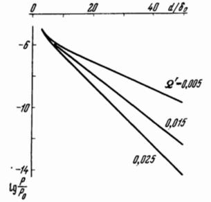
FIG. 3. Dependences of the maximum intensity of the microwave signal, transmitted at the antiresonance point, on the thickness of a sample for several values of the damping  $\Omega'$  ( $\Omega = 1.5$ ). The magnetic field is assumed to be parallel to the plane of the plate.
