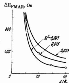
FIG. 8. Dependence of the FMAR line width ( $f = 36.6$  GHz) on the thickness of a sample. The field  $H$  was parallel to the plane of the sample. The continuous curves represent the theoretical dependences calculated for various values of the damping and  $\Omega = 1.5$ .
