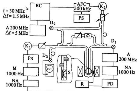
FIG. 5. Block diagram of the apparatus: S is a sample; PS is a power source; M is a modulator; NA is a narrow-band amplifier; A is an amplifier; PD is a phase sensitive detector; R is an X-Y automatic recorder; AFC is an automatic frequency control unit; RC is a resonance circuit;  $K_1$  and  $K_2$  are klystrons; and  $D_1$ ,  $D_2$ , and  $D_3$  are detectors.
