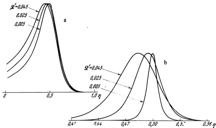
FIG. 4. Comparative curves showing the influence of the damping on the FMAR width: a)  $d/\delta_0 = 6$ ; b)  $d/\delta_0 = 40$ . These curves are calculated for  $\Omega = 1.5$  and an external magnetic field parallel to the plane of the sample.
