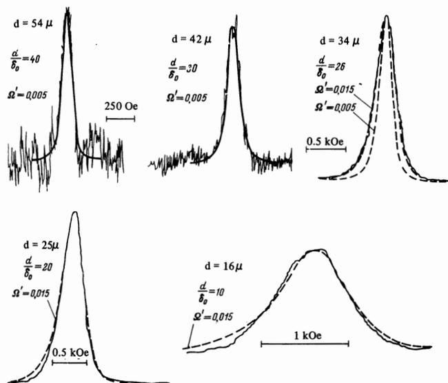
FIG. 7. Comparison of the observed ( $f = 36.6$  GHz) and calculated ( $\Omega = 1.5$ ) antiresonance line profiles obtained for various thicknesses of a sample. The magnetic field was parallel to the plane of the sample.
