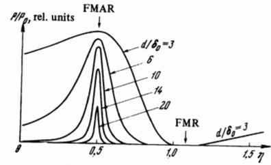
FIG. 2. Dependences of the transmitted microwave power on the external magnetic field, calculated for various thicknesses of a sample ( $\Omega' = 0.005$ ,  $\Omega = 1.5$ ). The magnetic field is assumed to be parallel to the plane of the plate.
