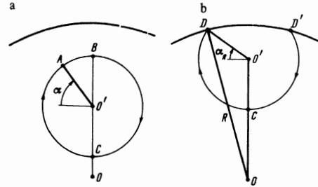
FIG. 2. Trajectory of an electron that does not collide (a) and collides (b) with the surface of the cylinder.
