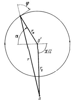
FIG. 1. Larmor trajectory of electron. O—cylinder axis. O'—center of Larmor circle.
