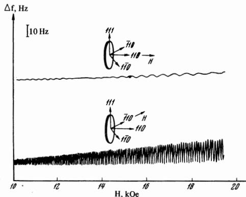
FIG. 2. Oscillations of the frequency of a helicon generator based on sample Al-1. The geometry of the various directions is shown in the figure. The monotonic component of the dependence of the frequency on the magnetic field, compensated by a signal provided by a Hall probe, increased from 300 to 520 Hz in the upper curve and from 150 to 260 Hz in the lower curve. Both curves show short-period  $\gamma$ -type oscillations and long-period  $\alpha$ -type oscillations (see [9]).
