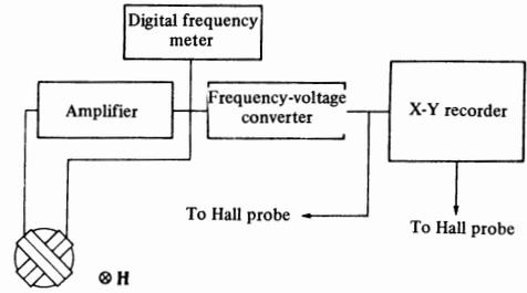
FIG. 1. Block diagram of the experimental set-up.
