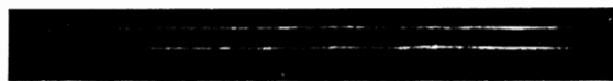
Self-focusing filaments in ADP crystal. Magnification 7X. The arrow indicates the direction of the incident beam.
