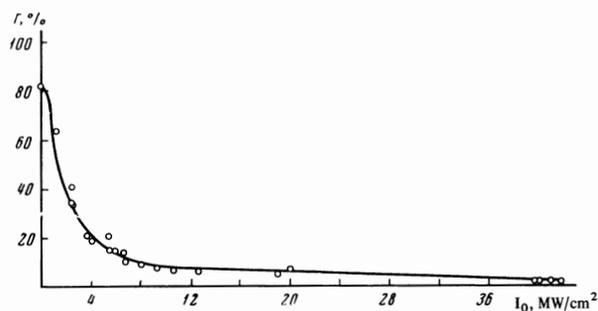
FIG. 2. Dependence of the transmission of the colloidal solution of phthalocyanine of aluminum chloride in dichlorobenzene on the intensity of the incident radiation. Points—experimental values, solid line—calculated curve.
