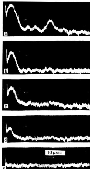
FIG. 5. Oscillograms of probing beam at different power densities of the laser radiation: a—40, b—30, c—25, d—18, e—9  $\text{MW}/\text{cm}^2$ .
