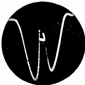
FIG. 5. Resonance curve of unmatched resonator in the oscillatory mode at the klystron generation band (narrow-band receiver).
