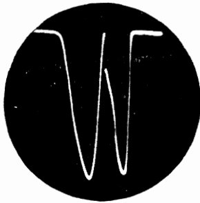
FIG. 1. Resonance curve of unmatched resonator in the klystron generation band; jumps of the reflection coefficient in the absence of oscillations of the reflection coefficient.
