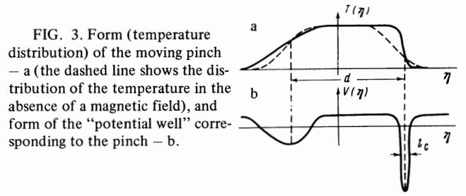
FIG. 3. Form (temperature distribution) of the moving pinch – a (the dashed line shows the distribution of the temperature in the absence of a magnetic field), and form of the “potential well” corresponding to the pinch – b.
