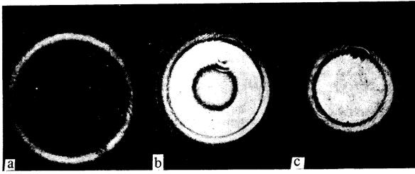
FIG. 3. Image in the focal plane of the lens for various crystal orientations: a – crystal turned  $10'$  from optimal position; b – crystal turned  $3'$  from optimal position; c – image at optimal orientation.
