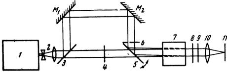
FIG. 4. Diagram of experimental setup. 1 – Nd glass laser; 2 – telescope; 3, 5 – K-8 glass plates;  $M_1, M_2$  – mirrors; 4 – image plane; 6 – resolution grid; 7 – KDP crystal; 8 – SZS-21 filter; 9 – NS-2 filter; 10 – lens; 11 – film.
