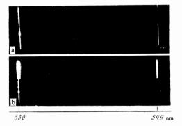
FIG. 3. Intensity ratio of the first Stokes SRS components scattered in the forward and backward directions, at different pump levels: a - second harmonic power 5 MW/cm<sup>2</sup>; b - 100 MW/cm<sup>2</sup>.
